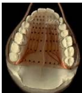
Figure1: The Reading EPG artificial palate similar to the one used in this study, and the plaster impression showing the position of the electrodes in the mouth (Hardcastle, et al. 1989: 3)
